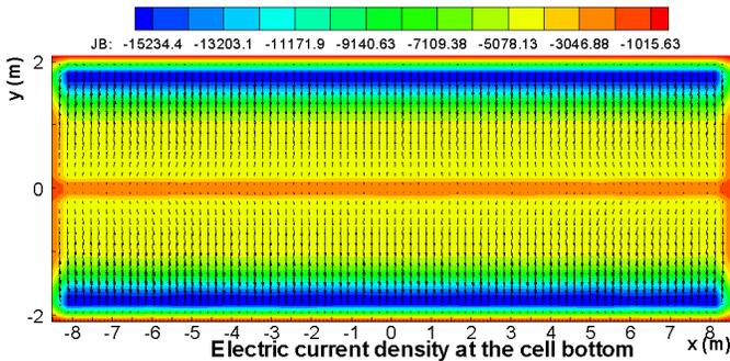
Figure 12. Current density solution on the top surface of the cathode in A/m<sup>2</sup>
