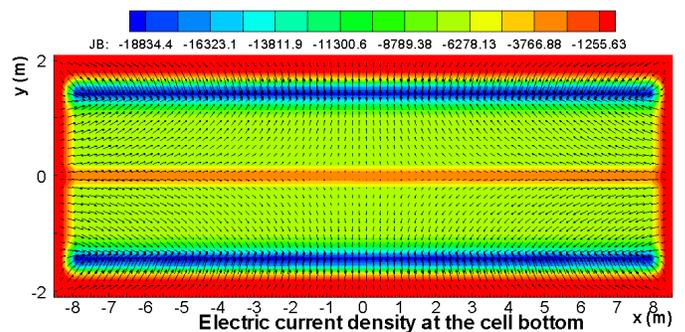
Figure 20. Current density solution on the top surface of the cathode in  $A/m^2$
